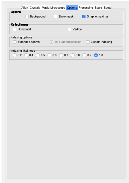
(a) Options to control the indexing process, in particular the number of spots used by the indexing.
