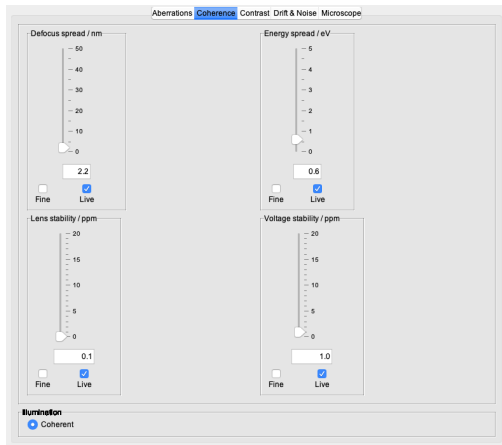
(a) Coherence settings of the microscope illumination.
