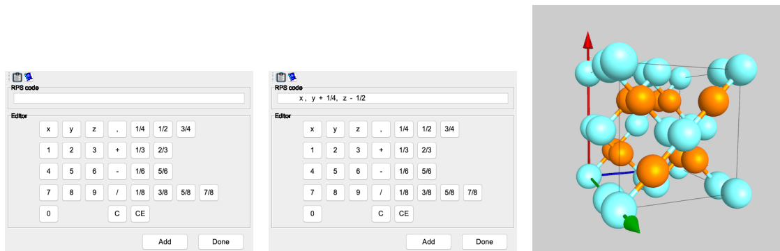
(a) RPS code editor dialogue. (b) Using the Editor keys (or entering the code directly) to define a new code (x, y + 1/4, z - 1/2) . (c) jems does not check the new code validity \rightarrow 3-D view of the updated unit-cell.
