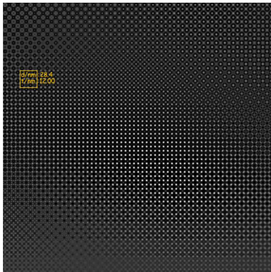
Figure: Fe_3S_4 HREM map Bloch-wave method (1 + 436 BW)
