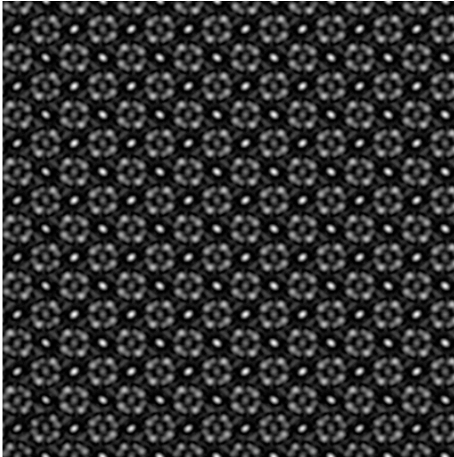
Figure: HRTEM image Cr_3Ni_5Si_2 [001] , thickness 10 nm, defocus -8.2 nm.
