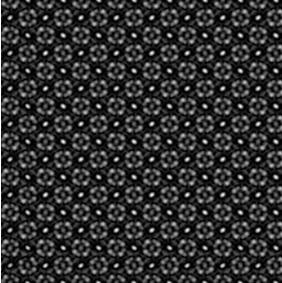
HRTEM image Cr_3Ni_5Si_2 [001] , thickness 10 nm, defocus -8.2 nm.
