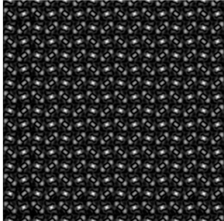
HRTEM image Cr_3Ni_5Si_2 [001] , thickness 10 nm, defocus 8.2 nm.
