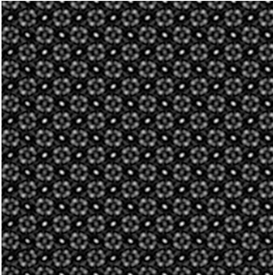
HRTEM image Cr_3Ni_5Si_2 [001], thickness 10 nm, defocus -8.2 nm.
