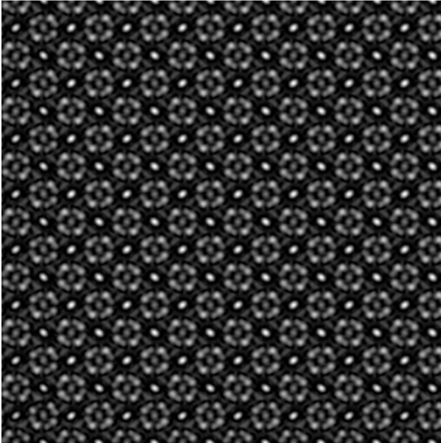
HRTEM image Cr_3Ni_5Si_2 [001] , thickness 10 nm, defocus -8.2 nm.
