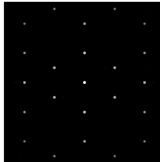
AlN: SAED diffraction pattern.
